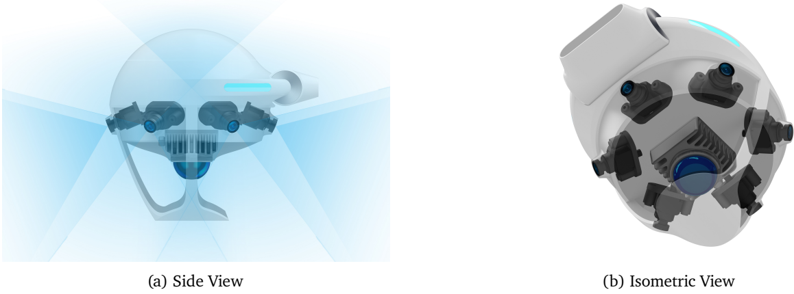
Figure 4: Structural visualization of humanoid occupancy hardware. We equipped the humanoid robot head with 6 cameras and a lidar to acquire sensory information. More details in Sec. 3.2
